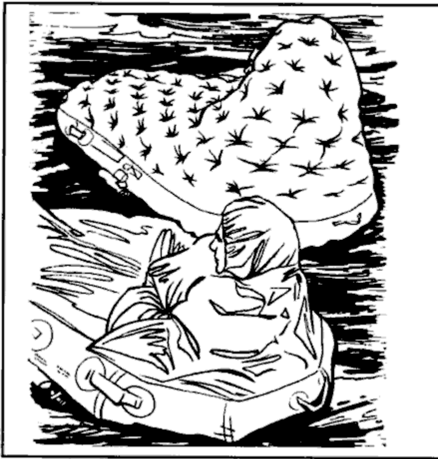
Figure 16-11. One-man raft with spray shield inflated.
